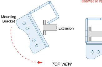
Tighten thumb screws to secure connection to inside of frame.
