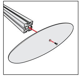
**Base Plate & Extrusion Connection**
