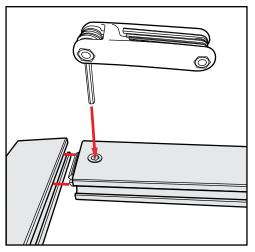
**Extrusion & Lock Connection**
